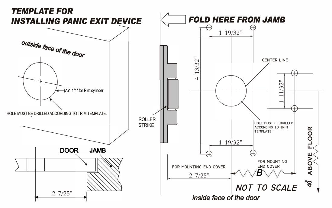
(A)For T341H07 Series (UL Listed)-Drill & tap for(6)1/4"×20 machine screws for Exit Device and Drill & tap for(3)1/4"×20 machine screws for Roller Strike. OPTIONAL for T341H07 (UL Listed)
