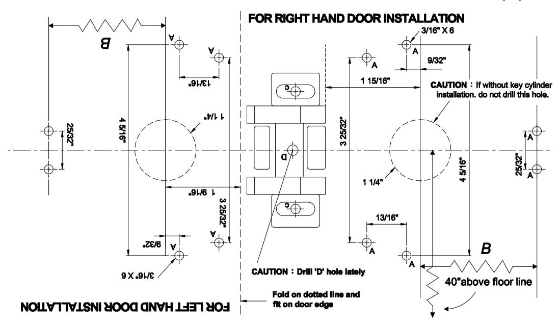
(A)For (UL Listed)-Drill & tap for (6) 1/4"x20 machine screws for Exit Device and Drill & tap for (3) 1/4"x20 machine screws for Roller Strike OPTIONAL for (UL Listed)
