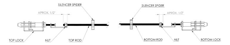
3. Place the rod assembly on the face of the door with the center mechanism aligned with the installation hole; and extend the rods fully.
