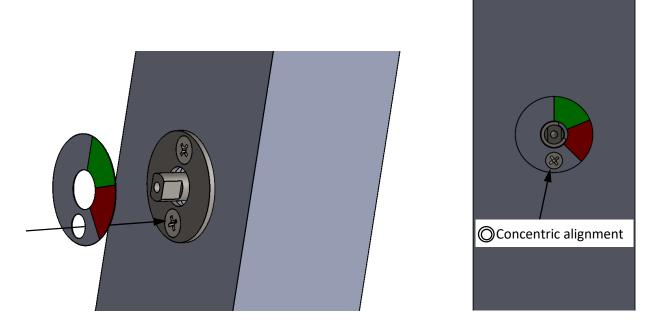
11. Position the knob by screwing it to the stem of the central mechanism using the W5/32"x1/2" screw.
