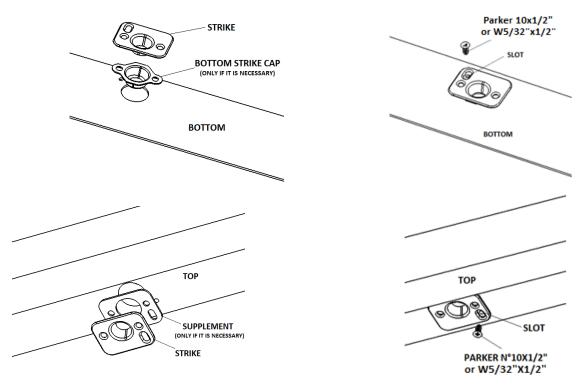
4. Once the position of both strikes (top & bottom) is defined, mark and drill the remaining 2 holes and fix the strikes with the 2 Parker screws N°10x1/2" or W5/32"x1/2" as shown in the image.
