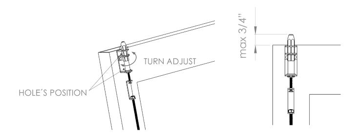
5. Adjust the bottom lock turning in clock or anti-clock side the bottom lock as shown in the picture (2 full rotations equivalent to 7/64" projection). The minimum recommended projection is 1/2"+gap (edge door with floor). The standard max projection its 3/4".
