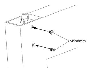
9. Secure the bottom lock with two (2) provided M5x8mm flat head screws.
