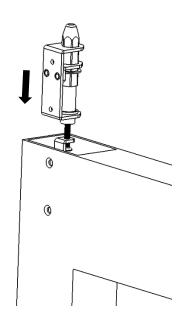
7. Align the central mechanism with the central inner hole, help yourself with the W5/32"x1/2" screw by screwing it to the central mechanism as shown in the image. Fix the assembly by means of the indicator washer and using the flat head screws M5x12mm. Remove the W5/32" screw once mechanism attachment is complete.
