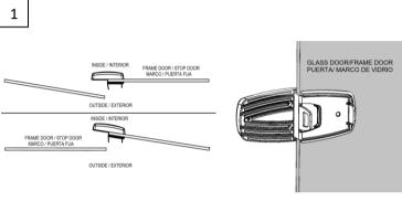
Place the rear part on the frame / stop door or on the swing door according to the opening direction of the door, as shown in the images (the indicated refers in the case that you want to close from the outside, in case of doing it from the inside, the installation direction should be
