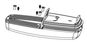
Remove the M4x10 screws with a PH 2 screwdriver, as shown in the image.
