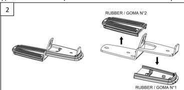
Remove the rubbers N ° 1 and N ° 2 from the Z plate, as shown in the images.
