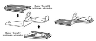
Place the additional rubbers N°1 and N°2 (for use on ½" thickness glass door), as shown in the images.
