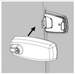
Before installing the front part, check that the latch is not activated, if it is, turn the key and deactivate it. Then place the front part on the back as indicated in the image and turn the key leaving the lock locked.
